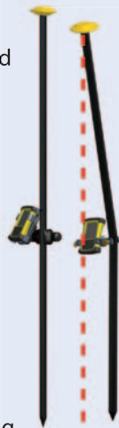
Error caused by bent pole
